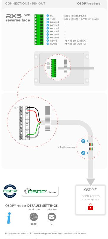
The RX5<sup>-WE</sup> is a Third Millennium styled flush Panel Mount reader. The unit is a multitechnology reader suitable to interface with all standard access control systems, and may be used in speed gates and turnstiles, or other third-party enclosures.
